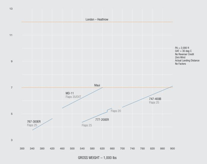
Overweight automatic landings are not recommended. Autopilots on Boeing airplanes are not certified for automatic landing above the maximum design landing weight.
