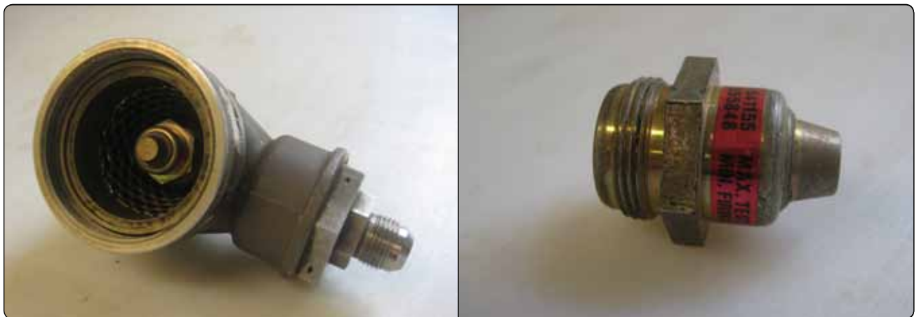
Figure 17-14. Discharge valve (left) and cartridge, or squib (right).
