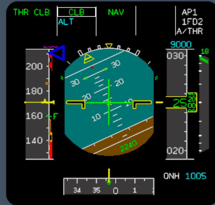
As SRS disengages (at Acceleration Altitude), on PFD speed target is 210 Kts shown as a selected blue ( ). CLB becomes the engaged mode and ALT becomes armed in Blue.
