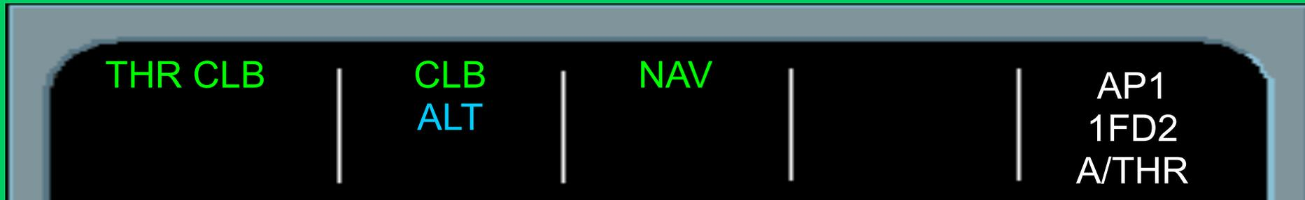
As the constraint is passed (we are in Managed Mode), Thrust goes to Climb Thrust (itself) and the aircraft resumes climb (itself). CLB becomes engaged mode and ALT armed, as FCU ALT is set at FL-290.
