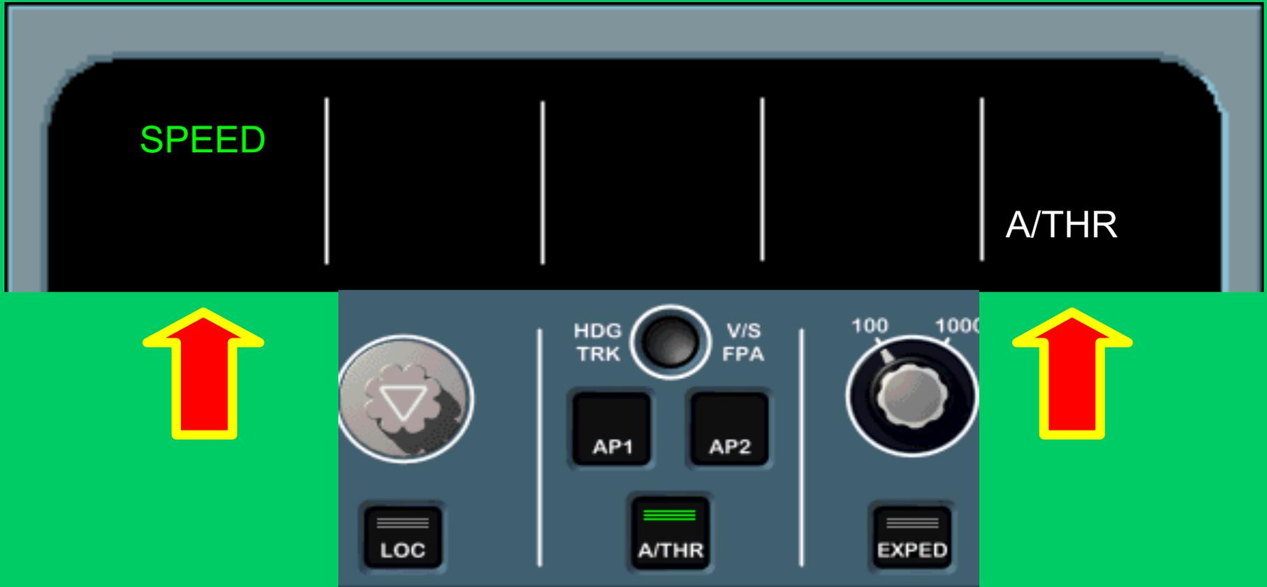
Normal Cruise conditions. Both FDs OFF. A/P is OFF. A/THR goes in SPEED mode. Lateral & Vertical column become blank. AP & FD indications go OFF.
