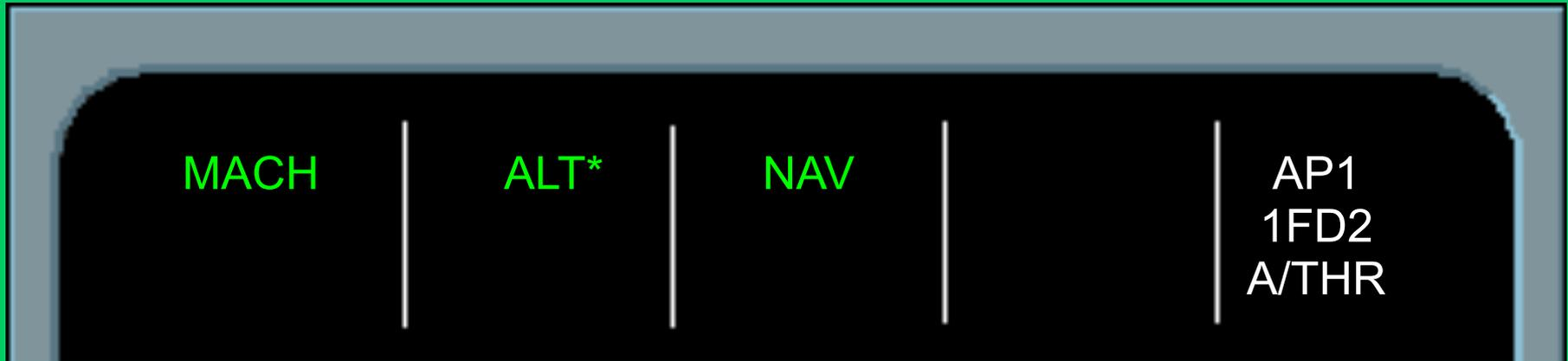
At ALT\* engagement, EXEP CLB automatically disengages.
