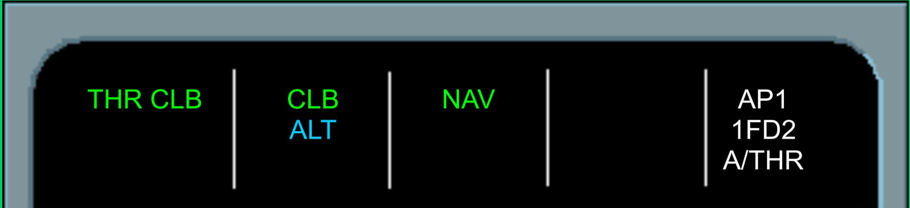
Push the ALT knob, SPEED changes into THR CLB, V/S into CLB and NAV remains as it is.
