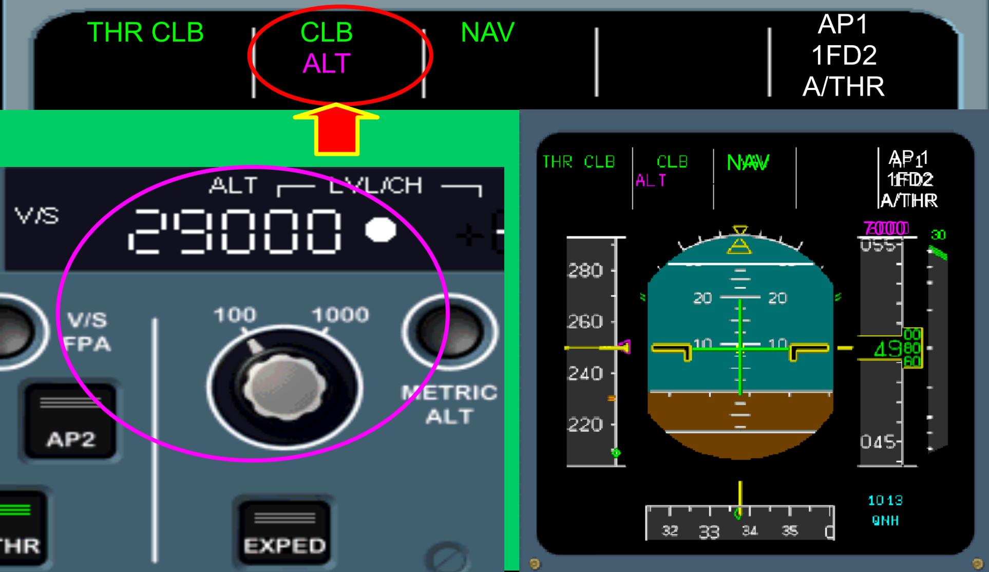
There is an Altitude Constraint at, say FL 070. ALT (in magenta) is the FMGC constraint. FCU ALT set at FL-290.
