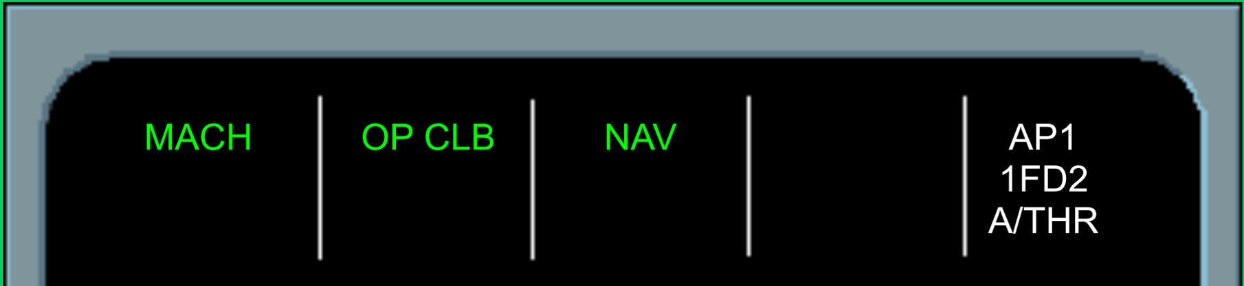
Pull the ALT knob on the FCU to engage Open Climb. You can also adjust the V/S to reach the desired level.
