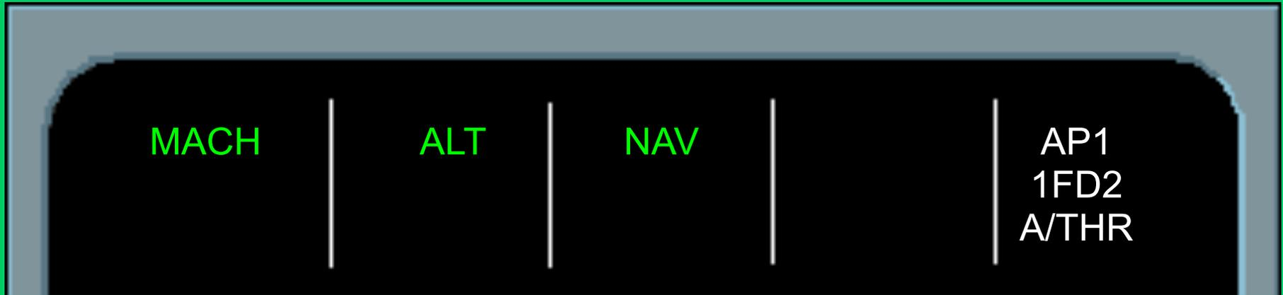
Above (ALT in Green) shows that the aircraft has leveled off at altitude **below** the FMGC entered altitude.
