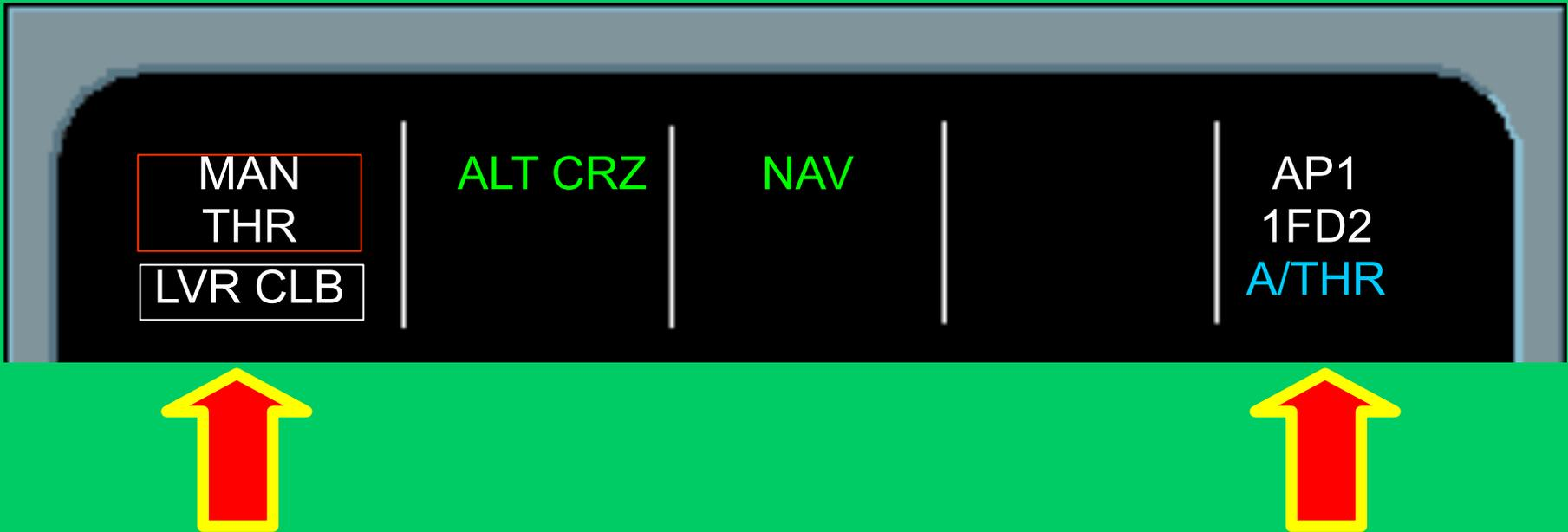
When both thrust levers (AP-BRJ) are moved ahead of Climb Detent, “MAN THR” in steady white with Amber box, and “LVR CLB” flashing. Advising Pilot to Set Thrust Lever to Climb Detent. A/THR becomes BLUE i.e. armed.
