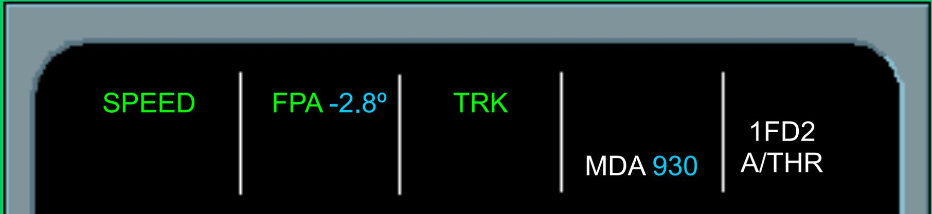
When A/P is disconnected or happens automatically at MDA -50 feet or at 400 ft if no MDA entered.
