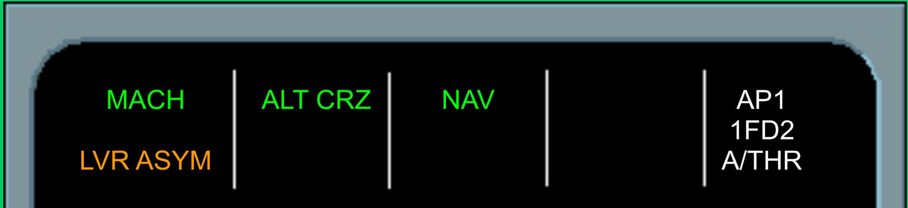
In a Normal Cruise (AP-BRJ) if one Thrust Lever is moved below the Climb Detent **LVR ASYM** in steady amber. Set the Thrust Lever in climb detent. A/THR is Active (White).
