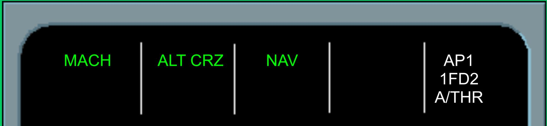
In a Normal Cruise, the FMA is as shown above. Both Thrust Levers are in Climb Detent. A/THR is Active (white).
