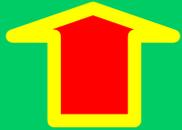
Auto Thrust active and TOGA Thrust is locked. "Alpha Floor" conditions are no more met. Pilot must disconnect A/THR.
