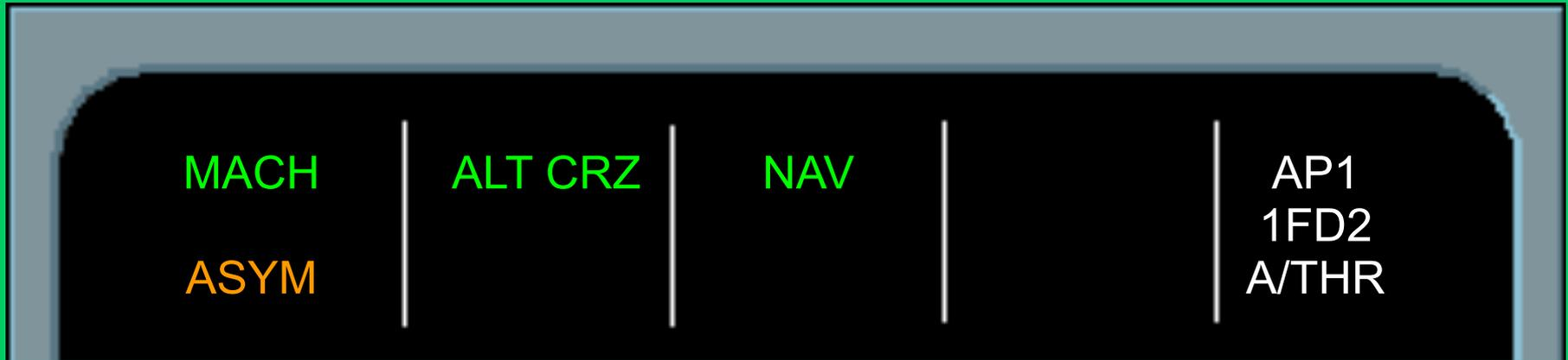
In some aircraft (AP-BGU & AP-BGV) if one Thrust Lever is moved below the Climb Detent **ASYM** in steady amber. Set the Thrust Lever in climb detent. A/THR remains Active (White).
