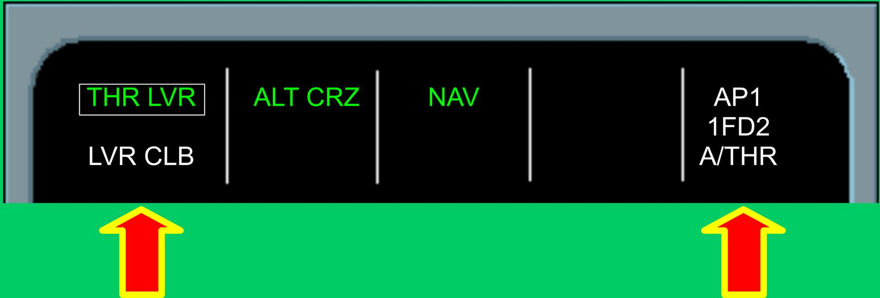
If one Thrust Lever (AP-BRJ) is moved ahead of the Climb Detent, THR LVR in Green with a white box.
