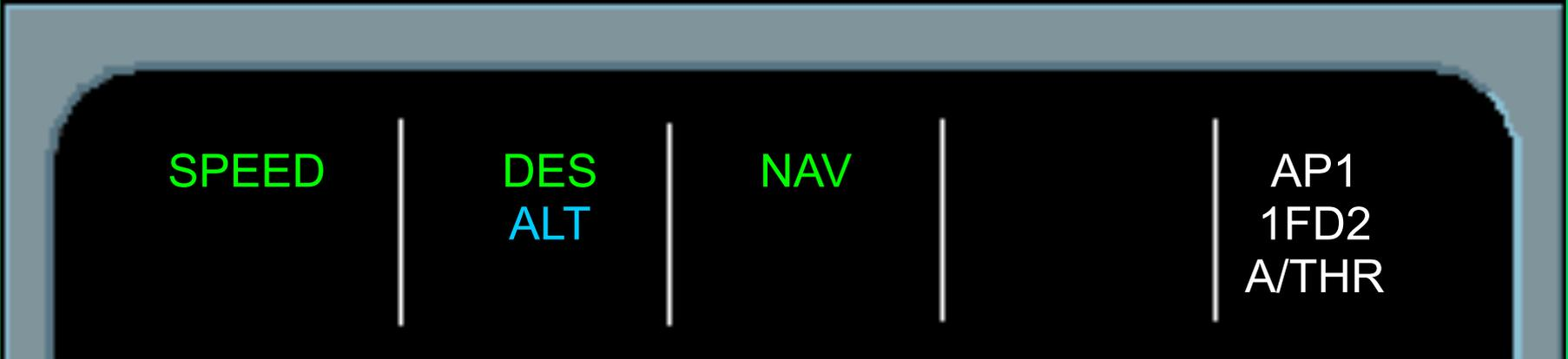
THR IDLE changes to SPEED. Thrust is added to get the higher speed. As DES is engaged, the VDEV remains zero. The speed triangle on the speed tape is selected blue (
