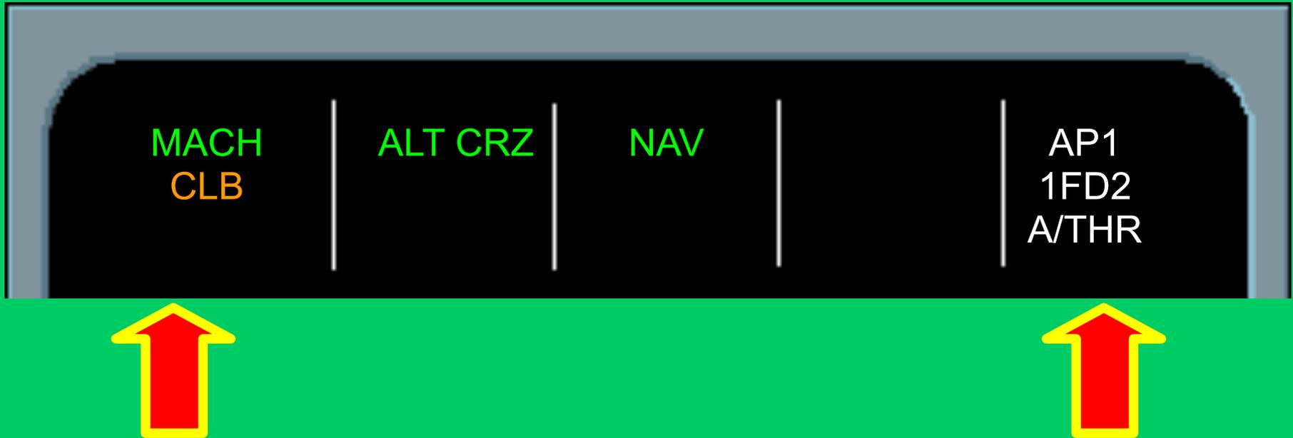
In some aircraft (AP-BGU & BGV), when both thrust levers are moved below Climb Detent, “CLB” in Amber Flashes. Advising Pilot to Set Thrust Lever to Climb Detent.
