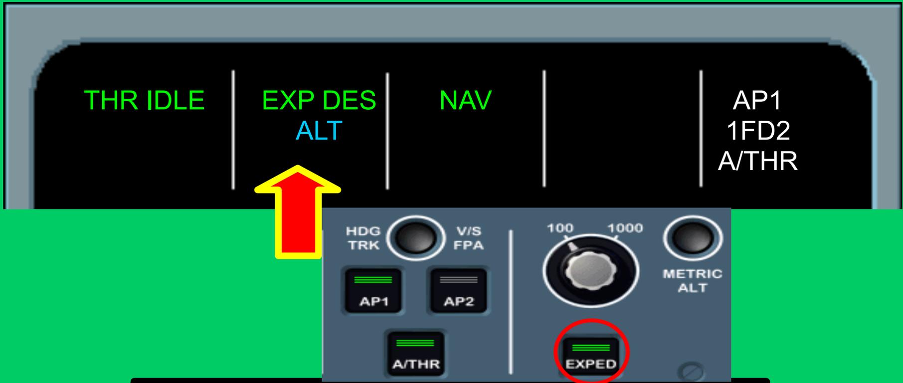
When EXPED P/B on FCU is pushed, EXP DES in Green. Target speed 340 Kts / 0.8 Mach.
