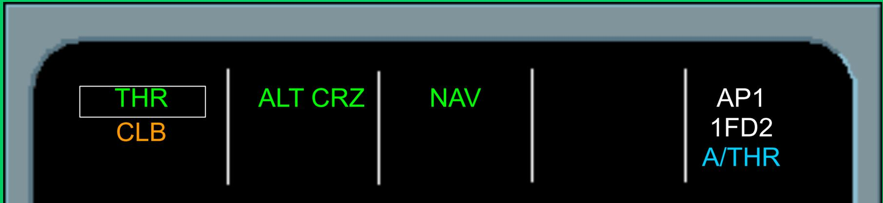
In some aircraft, (AP-BGU & BGV) both thrust levers are moved ahead of Climb Detent, “THR” in Green steady with a white box, with “CLB” in amber flashing. Advising Pilot to Set Thrust Lever to Climb Detent.
