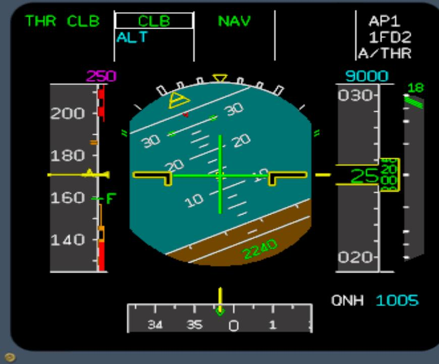
In case you want to revert to the Managed Speed, push the Speed knob on FCU. On PFD speed target goes to 250 Kts shown as a Managed Magenta ( ). CLB remains the engaged mode and ALT remains armed in Blue.
