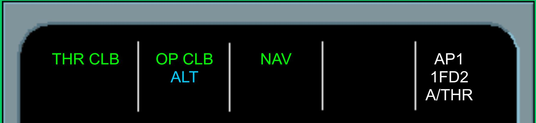
Pull the ALT knob, SPEED changes into THR CLB, V/S into OP CLB and no change in NAV.
