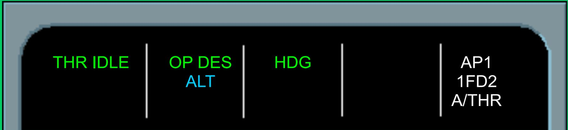
Thrust will be THR IDLE. The speed triangle on the speed tape is managed magenta ( ). However, during managed descent it is an open bracket with a speed range of  $\pm 20$  Kts.
