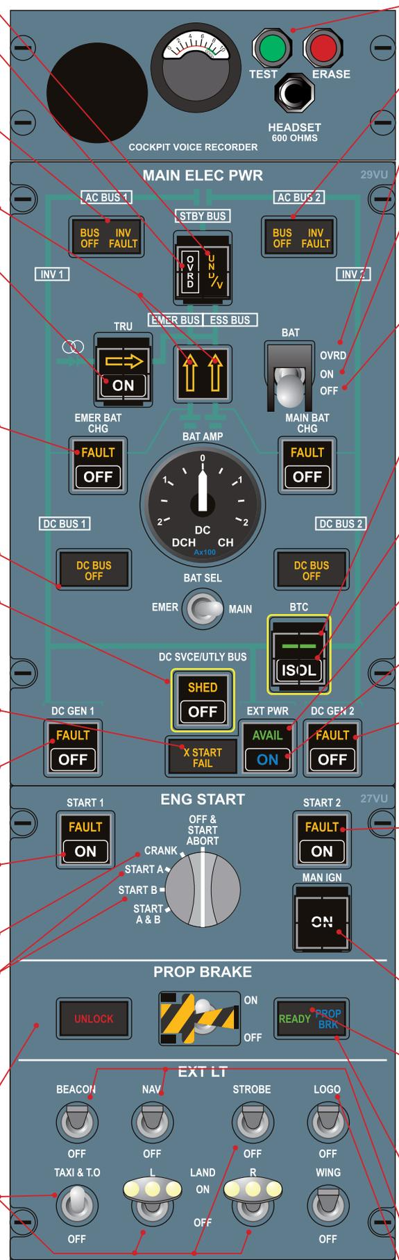
On external power, pedestal PB must be on to power CVR test
