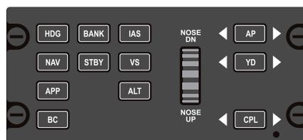
Mode selection is achieved by acting on the corresponding PB on the AFCS control panel except for ALT SEL and GO AROUND modes.
