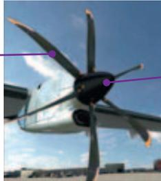
Spinner: secure, spinner indicator aligned with propeller indicator, no impact
