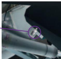
Beacon: condition, glass not broken and flashing if selected ON
