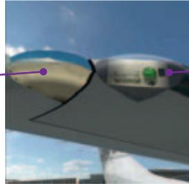
NAV and strobe lights: condition, glass not broken, and NAV illuminated if ON
