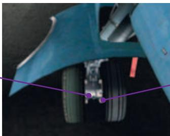
Brake wear detectors: check indicator out of bolt
