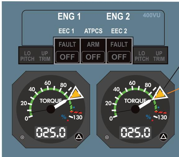
The go-around torque is read in the QRH, Ops Data part.
