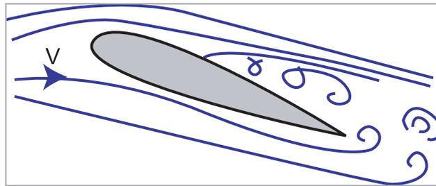
The secondary stall is a premature increase in angle of attack that results in another stall event during stall recovery, prior to establishing stable flight conditions.
