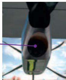
Flaps position: check the position in accordance with the flaps lever
