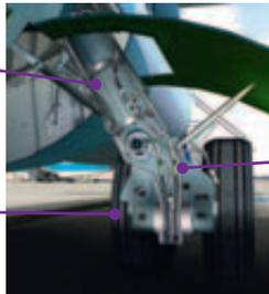
Wheels and tires: condition, no crack, inflation
