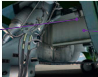
Wheel well: condition, no leak
