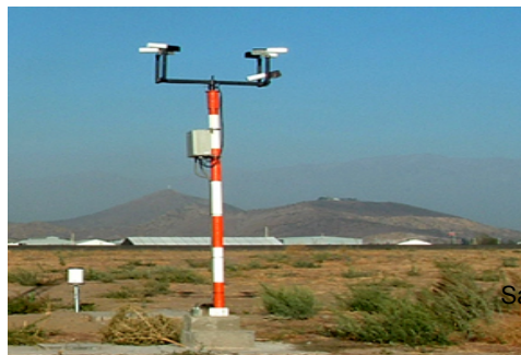
Vaisala MITRAS 18 Transmissometer sensor mast and array (Vaisala company Oyj, PO Box 26 00421 Helsinki, Finland)
